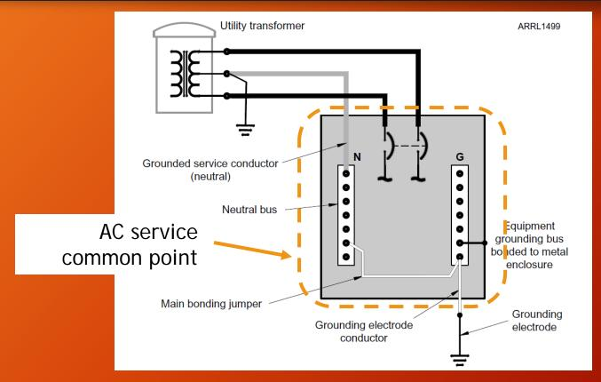
Grounding and Bonding for Home and Mobile HF Stations - 2021
