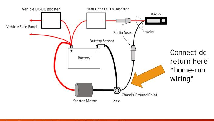
Grounding and Bonding for Home and Mobile HF Stations - 2021
