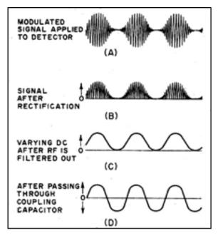
The simplest form of an AM receiver is a *diode detector*. Some of you built (or have seen) a crystal radio. A crystal radio has some form of inductor/capacitor-tuned network connected to an antenna (usually a random wire) to capture the desired signal's RF. That RF is a carrier (usually in the 500 KHz to 1.5 KHz AM broadcast band) modulated with voice or music (usually in the much lower 1KHz – 10KHz audio range).
