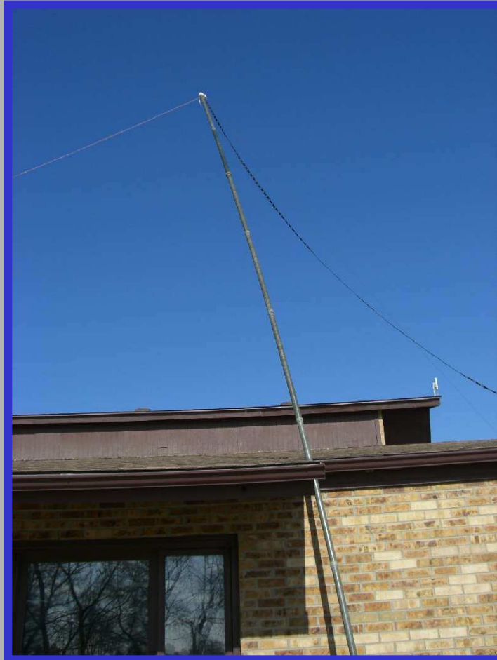
G5RV-type multi-band HF antenna. Fiberglass pole support.
