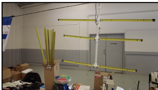
Yagi Fox Hunt Antenna Kits built by LARC being sold as a fundraiser for our club.
